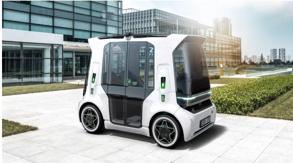
light is the Schaeffler Intelligent Corner Modules. In the four wheel modules, all drive and chassis components including the electric wheel hub motor are combined in one space-saving unit.
