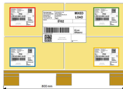
Fig.3 Example usage of the MIXED LOAD label on a non-homogeneous pallet (1200x800)
